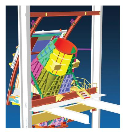
SDS/2 Fabricating is a solution designed specifically to meet the needs of fabricators. Fabricators simply request the model from the detailer, then can view the 3D model and 2D drawings, while having full control over the creation of CNC and MRP information necessary for the shop. Users may also use SDS/2 Fabricating's reporting and status tools to track the project through completion.
