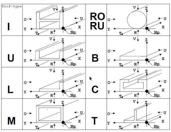
V = Web=front face U = Bottom O = Top H = Behind Np = Zero Point T = Displacement Direction
