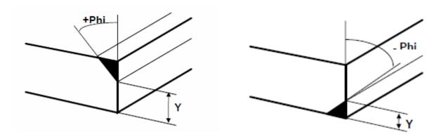
Bevels are defined along a edge of the piece as Negative or positive, and the depth provided for the bevel is as shown for each.
